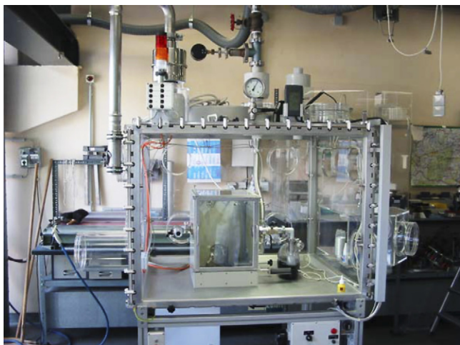
Fig. 4. Glove-box for handling of nuclear material, equipped with a fuming chamber for visualising fingerprints using the cyanoacrylate method.
